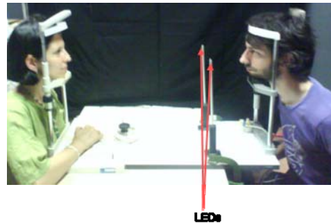
Fig. 6: New experimental set-up in which the to-be-responded target (LEDs) is visible by both the participant (on the left) and the experimenter (on the right).
