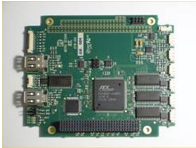
Fig. 21: The CFW (quad-can, firewire, sound) interface card that is installed in the head of the iCub. This card together with a standard Pentium-duo CPU makes the interface of the robot hardware with the external world by reading sensors and sending commands to the actuators.
