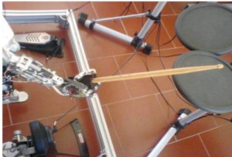
Fig. 15: iCub grasping the drumstick, and hitting the drum pads
