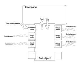
Fig. 1. The port internal structure: in practice either input or output connections, but not both, are used for a given instance of a port object.
