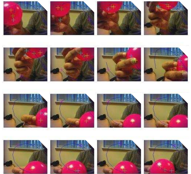
Fig. 3. Series of consecutive images from the Aibo camera showing ball path prediction using a sensorimotor interaction history. The robot does not move its head in this sequence. Images are sequential left to right and top to bottom and 147 images (73 experiences horizon length 40) precede these. The line shows the path prediction for 10 timesteps ahead. The crosses are from various methods for ball detection, only one of these was actually used as sensory input. Horizon=40, Number of Bins=5, Experience granularity=5 timesteps. Images captured approximately once every 2-3 timesteps.
