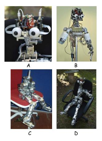
Figure 9. The ICub at various stages of construction. Panel A) shows the head of the robot with part of the embedded electronics and sensors; in B) the upper torso showing also the left hand; C) shows a first realization of the legs (now improved); D) a tentative assembly of the entire robot.
