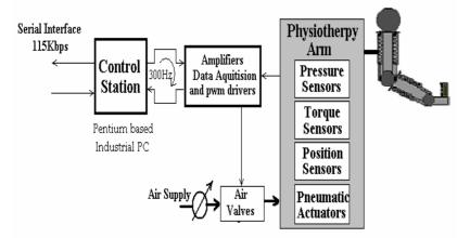
Figure 5. Control and interfacing hardware
