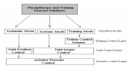
Figure 7. Layered control scheme and physiotherapy operation modes of the device.
