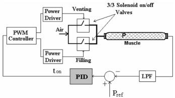
Figure 6. Control scheme of the muscle pressure using on/off solenoid valves
