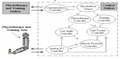
Figure 8. Object-oriented implementation of the device control.
