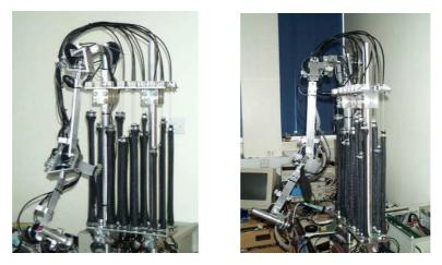
Figure 4. The system developed with the pneumatic muscle actuators.
