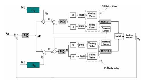
Figure 9. Block diagram of a single joint position or torque control scheme.
