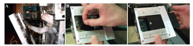
**Figure 1.** Experimental setup. A: Lateral view of the behavioral apparatus, requiring the monkey to perform a reach-to-grasp task. B: Demonstration of the precision grip the monkey had to execute in order to open the door of the food container. C: The target door was covered by an outer sliding door that the experimenter opened at each trial onset, giving the monkey a go-signal to start moving the hand from the resting position.
