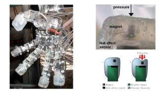
**Fig. 1.5.** Picture (left) and schematics (right) of the touch sensors mounted on the hand of James. Each fingertip has a couple of sensors based on a Hall effect technology. Eight more touch sensors are mounted on the phalanxes.
