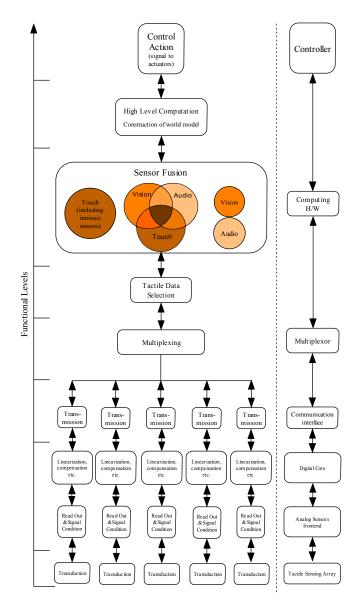
Fig. 1. Hierarchical functional and structural block diagram of Robot tactile sensing system.
