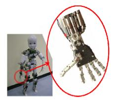
Fig. 2 Humanoid robot, 'icub' with the hand shown in inset.
