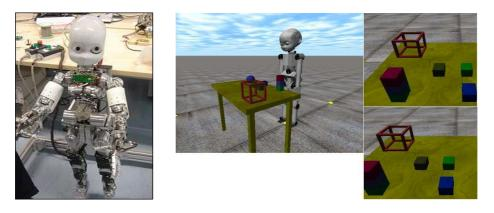
Figure 1: Photo of real iCub (left), of simulated iCub (centre) and of simulated robot's binocular view (right).
