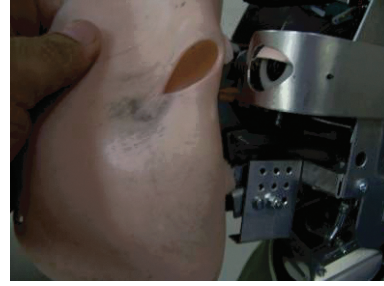
Figure 7. Detailed view of face mask attachment points.
