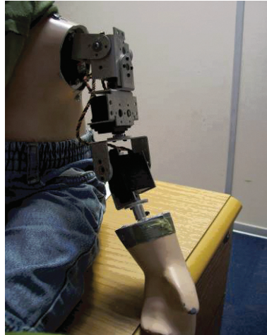
Figure A7. Arm is attached at shoulder end by plates fixed in the dummy body.
