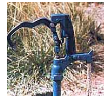
(b) Lever in ON position
