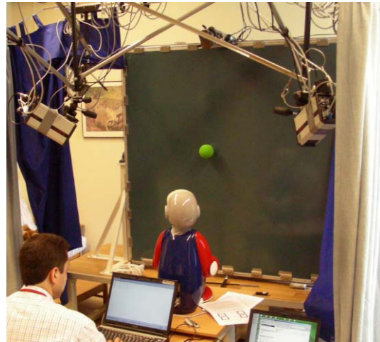
The iCub head following targets while the head-eye motion is being recorded.
