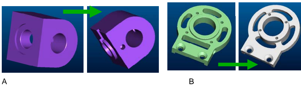
Figure 3: Examples of the changes required to two of the pulleys in the shoulder joints.
