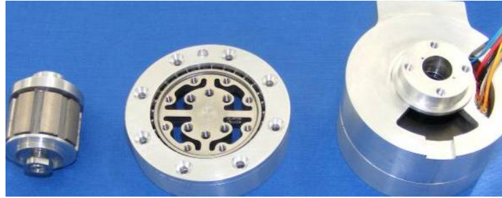
Figure 50: Section of the 3D mechanical assembly and mechanical parts of the updated motor/gearbox group.
