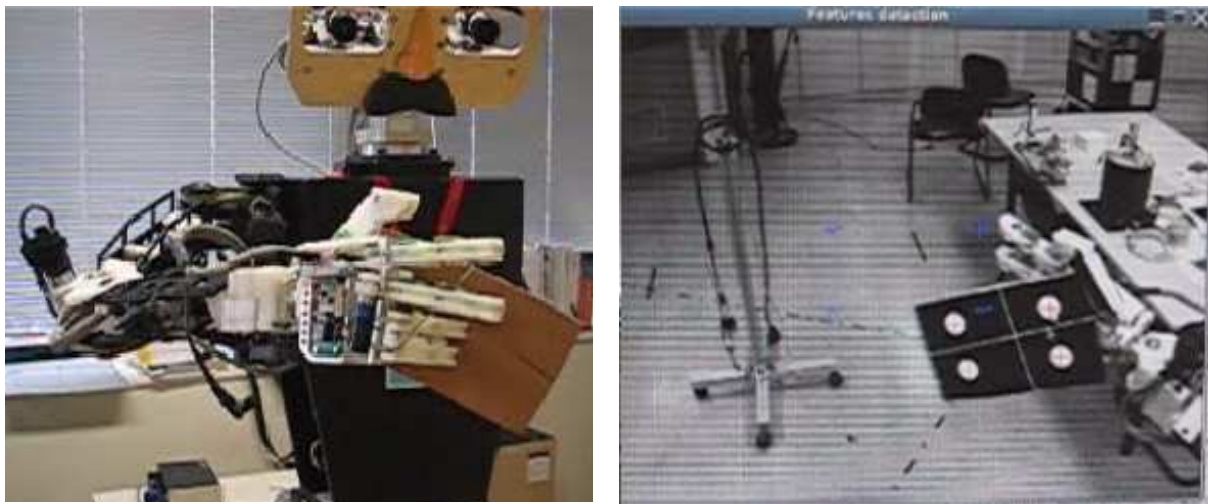
Figure 11: Left: Baltazar grasping an object using the learned VMM (both static and dynamic). Right: the view from one of Baltazar's cameras.
