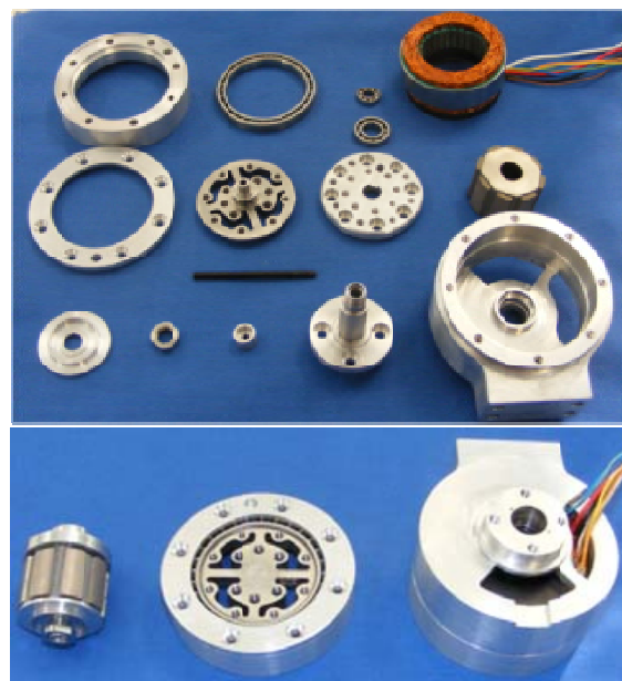
Fig. 4 Spare parts of the “iCub” motor/gearbox actuator group.
