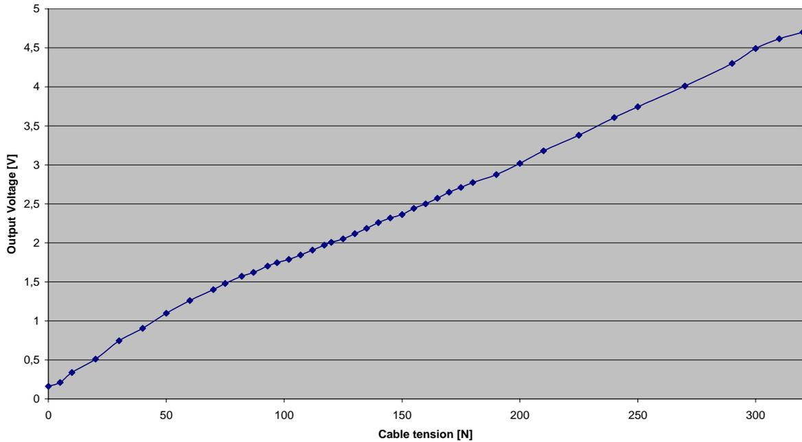
Fig. 2.4. The output of the sensor (alternative design)
