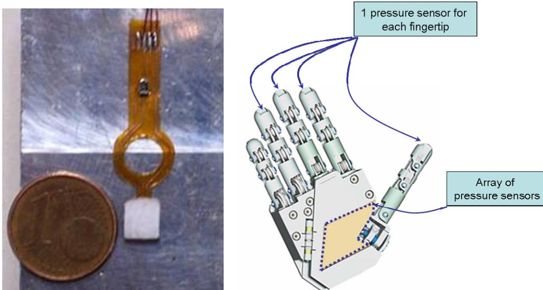
Fig. 2.7. The sensor developed and where it is placed in the hand
