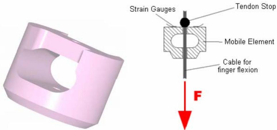
Fig. 2.3 Operating description of the tensiometer.
