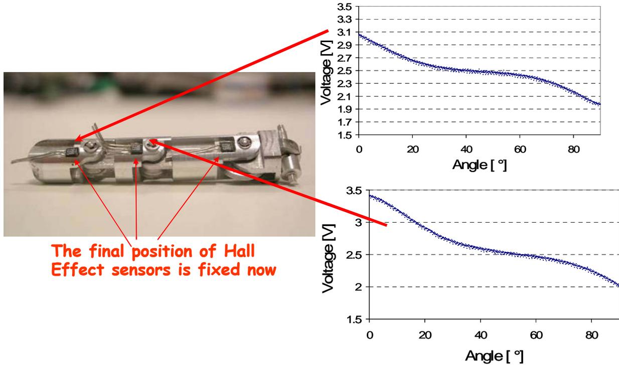
Fig 2.2 The artificial sensory system implemented
