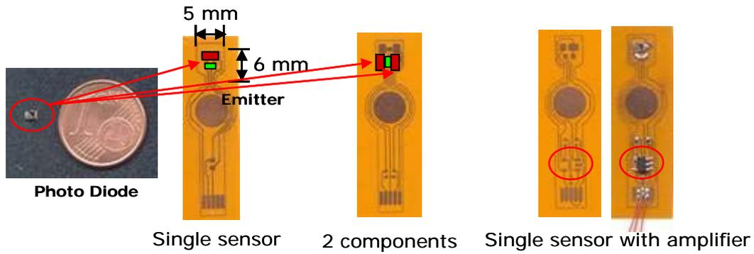
Fig. 2.8. The progressive development of the optoelectronic contact sensor. The electronic scheme is a simple comparator
