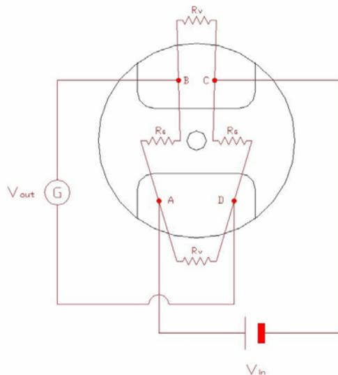
Fig. 2.5. The electric scheme of the sensor
