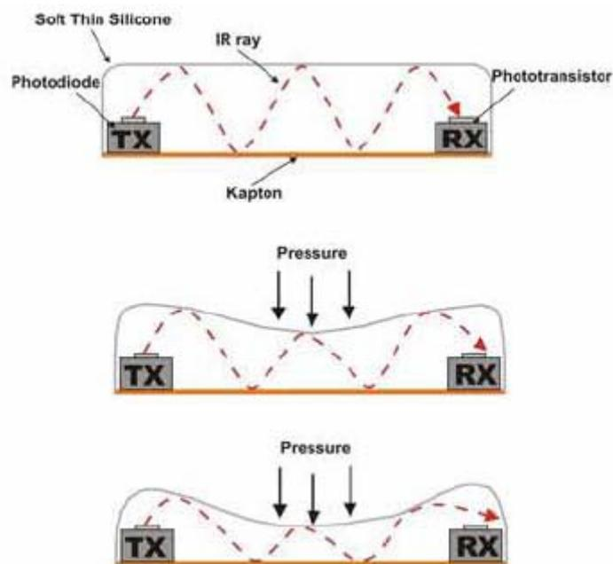
Fig. 2.6. The functioning principle of the developed optoelectronic contact sensor
