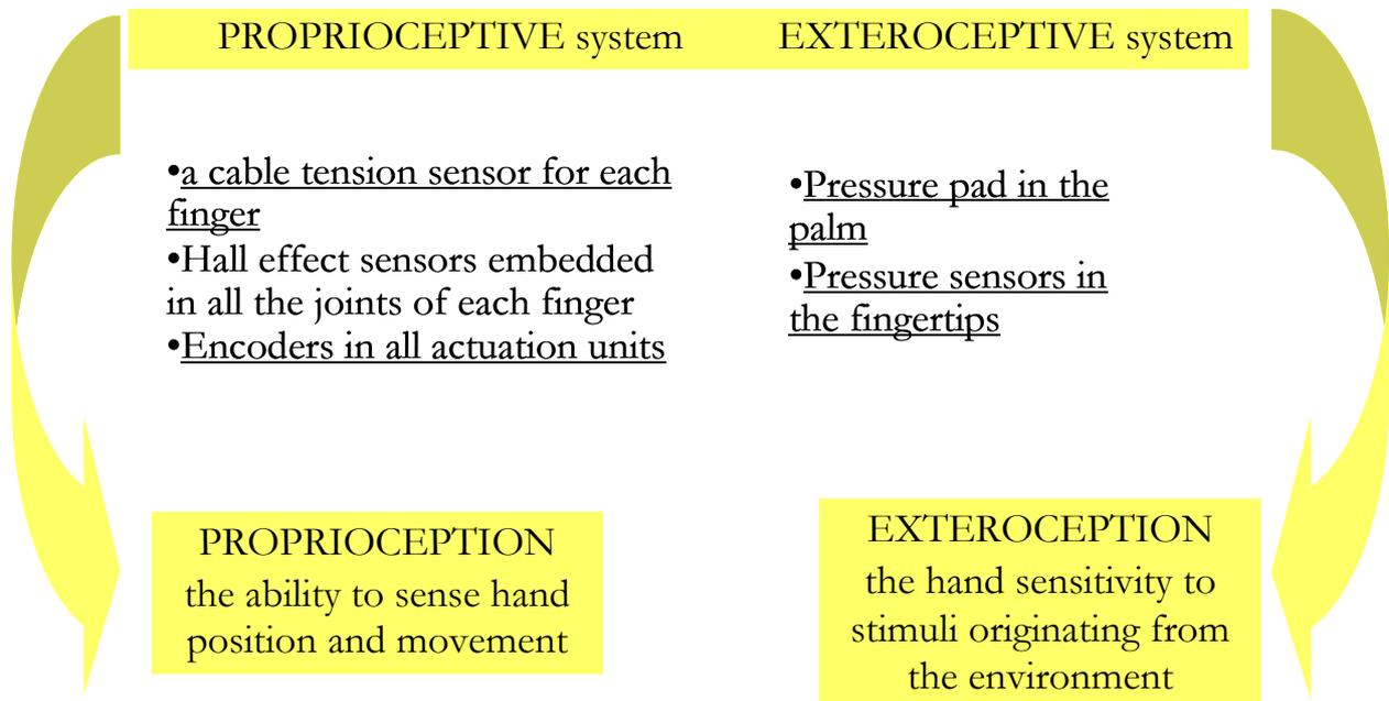
Fig 2.1 The artificial sensory system implemented.
