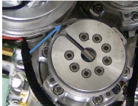
Figure 16: Shoulder tendon. The picture shows the point where two tendons tend to slide one over the other. This usually corresponds to an high friction which corrupt the tendon until its breaking.
