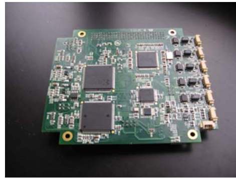
Figure 5: The new PC104 interface card with 10 CAN bus ports (see connectors to the right side of the PCB).
