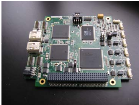
Figure 5: The new PC104 interface card with 10 CAN bus ports (see connectors to the right side of the PCB).
