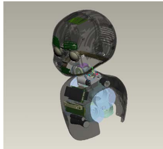
Figure 3: Details of the differential design of the neck (v2.0) and head assembly on the upper body.
