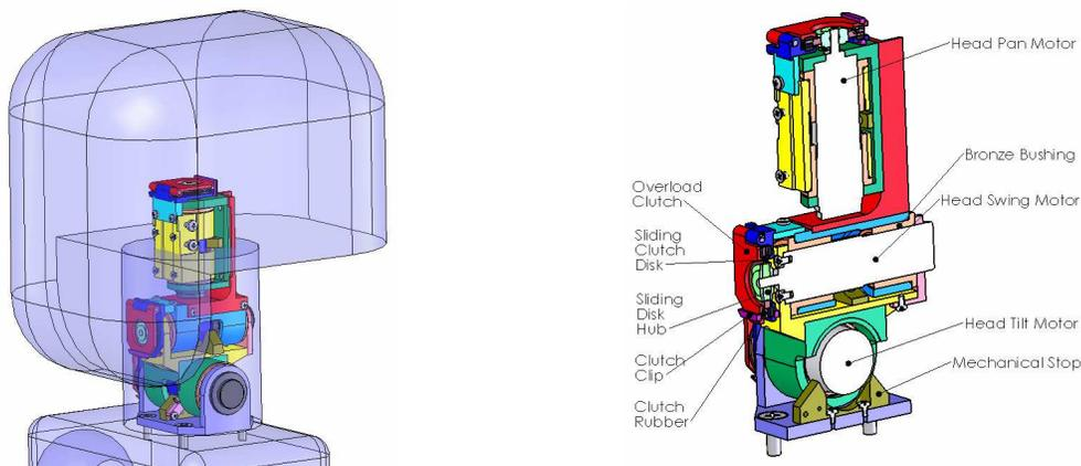
**Figure 6: The neck mechanism.**
