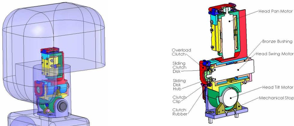
**Figure 6: The neck mechanism.**
