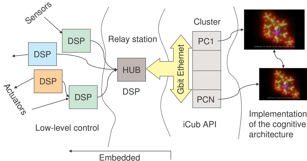
Figure 10: Levels of the hardware of the iCub.
