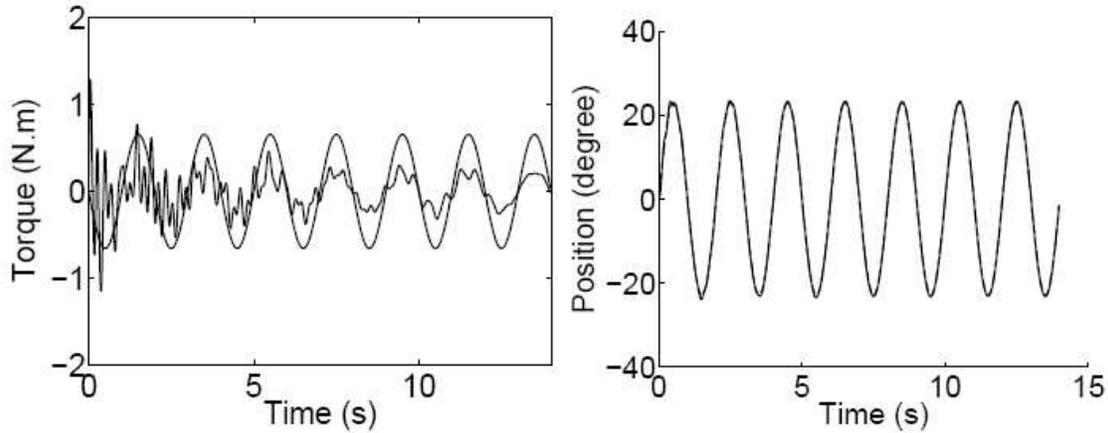
Figure 2: Torque applied to control the arm (left) and position of the arm (right). The right display contains both real position of the arm and of the desired position (input of the PID), we clearly see that they match very well (since we cannot distinguish them).
