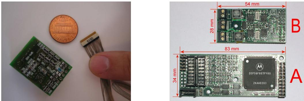
Figure 11: Left, ADC card. Right, motor controller card (A processor card, B amplifier card).
