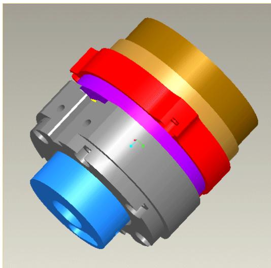
**Figure 4: The Kollmorgen motor and Harmonic Drive gearbox.**
