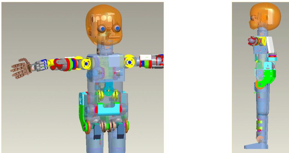
Figure 5: CAD drawing of the latest iCub.
