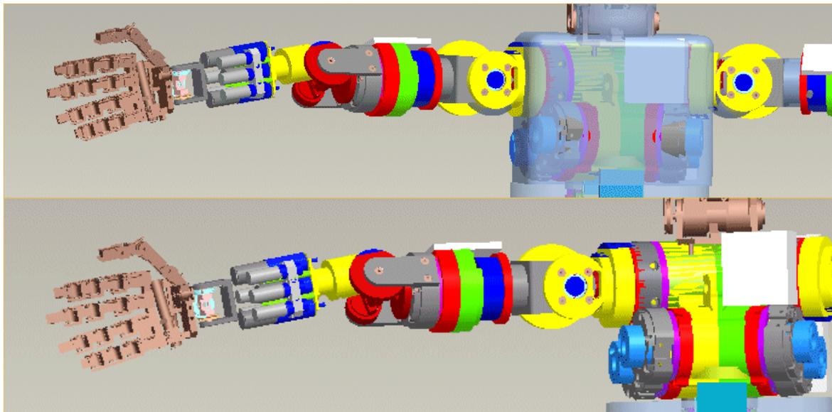
**Figure 8: One of the latest design of the arm subsystem with and without the external shell.**
