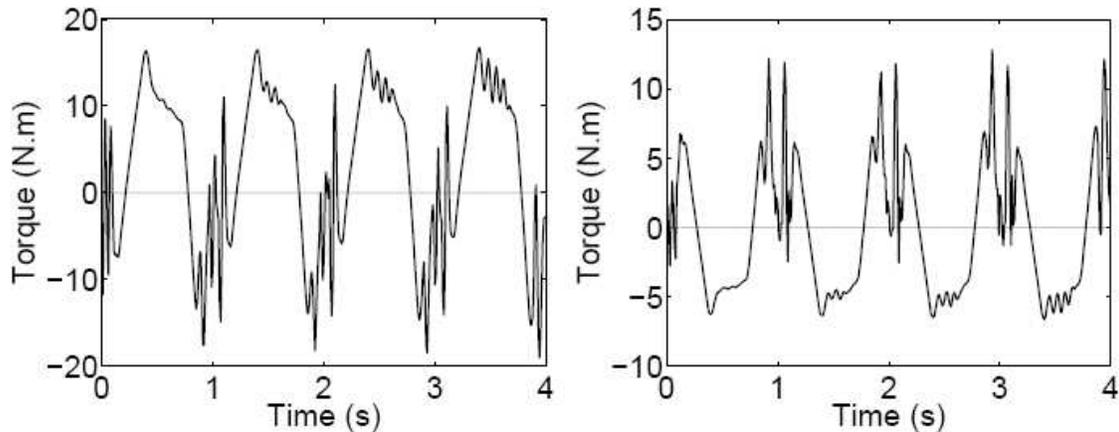
Figure 3: The left plot shows the torque applied to control the "left arm 2" joint. The right figure is a plot of the torque applied to control the left elbow.
