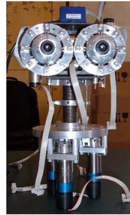
Fig. 4. Prototype of robot head with spring-based neck.
