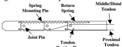
Figure 1 Tendon routing through the finger
