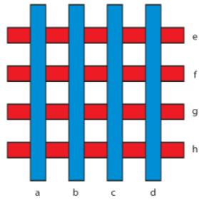
Figure 8 Skin sensor geometry configuration of the gauges
