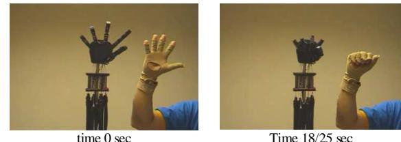
Figure 4 Total time from fully open to close is 0.72 sec
