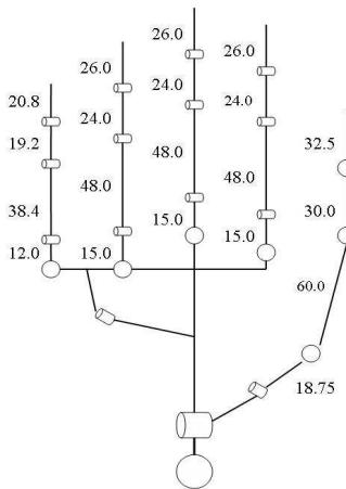
Figure 6 Kinematic chain of the 24 DOF hand
