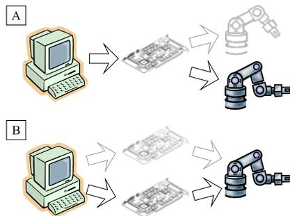
Fig. 3. YARP makes a distinction between *proximate* devices, such as control boards and framegrabbers which are used to talk to *distal* devices such as arms or sensors. In different systems, the same *proximate* device may be used to interface with different *distal* devices (A). Conversely, a given *distal* device may be interfaced with using a choice of *proximate* devices (B). Taking care to disentangle these two devices aids code reuse.
