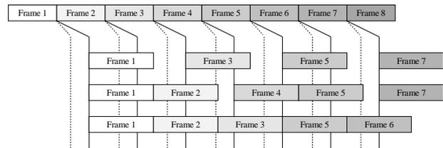
Fig. 2. The top row represents an output port configured for *no-wait*; dashed and solid lines show (exaggerated) start and end times of sending an update to three observers (input ports), configured as *single-buffer*, *double-buffer*, and *triple-buffer* respectively. For the scenario shown, the processing time of the client is greater than that of the server.
