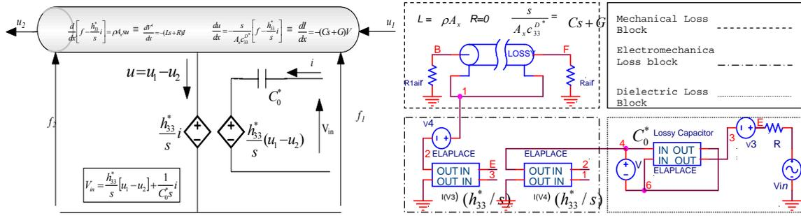
Fig 1: Piezoelectric polymer model and its implementation in PSpice. Here,  $h_{33}^*$  is the piezoelectric constant,  $u$  is the particle velocity,  $f$  is the force and  $s$  is Laplace operator,  $c_{33}^{D*} = c_{33}^D(1 + i \tan \delta_m)$  is the elastic constant,  $\epsilon_{33}^{S*} = \epsilon_{33}^S(1 - i \tan \delta_e)$  is dielectric constant and  $k_t^* = k_t(1 + i \tan \delta_k)$  is electromechanical coupling constant.
