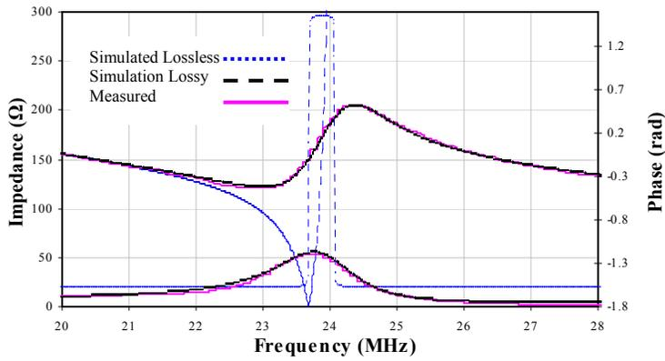
Fig 2: Comparison of Impedance and phase of a PVDF-TrFE sample ( $t = 50 \mu\text{m}$ ,  $A_x = 7 \text{mm} \times 7 \text{mm}$ ,  $\rho = 1880 \text{ Kg/m}^3$ ) around fundamental resonance. The simulated plots under lossless and lossy conditions have been compared with measured data. The impedance and phase were measured by HP4285A LCR meter.
