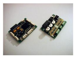
Figure 4: the brushless motor control logic and power amplifier of the iCub. Transistors and heatsinks are not shown. The size of the two PCBs is 58x42mm.
