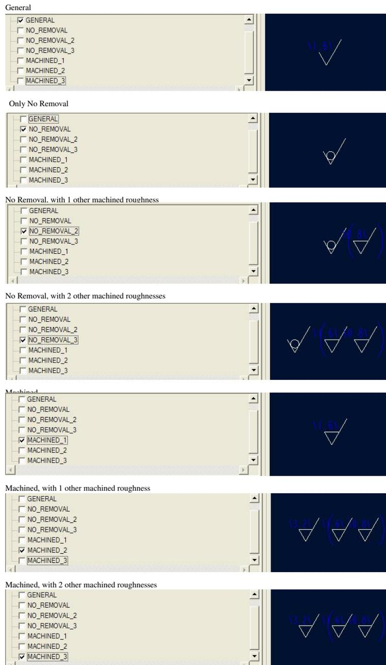
In all cases the symbol must be completed before its insertion with the “Var text” value. For roughness symbol in the drawing, the Pro/ENGINEER standard symbol (“isosurftext.sym”) in the “System Sym” directory should be used.
