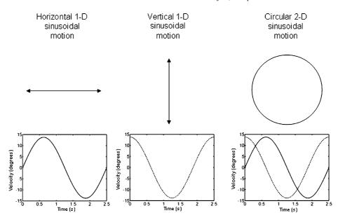
Fig. 2. The different object motions used in the experiment. The top row of figures shows the trajectories of the object. The bottom row shows the velocity profile of the motion.
