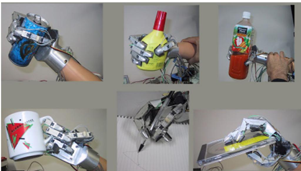
Figure 18 From upper left hand to the right: (a) grasping cylindrical form, (b) grasping elliptical form, (c) grasping a plastic bottle, (d) holding a coffee cup, (e) holding a pen, and (f) holding a CD case.
