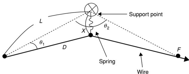
Figure 9 Adaptive joint mechanism mathematical model (Ishikawa *et al.* 2000).
