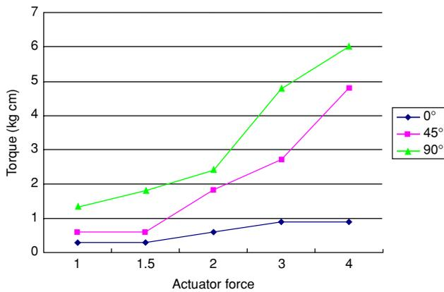
Figure 15 Statistics for the adaptive joint mechanism for the torque–actuator force relationship when substituting the spring for the spring coil wire.
