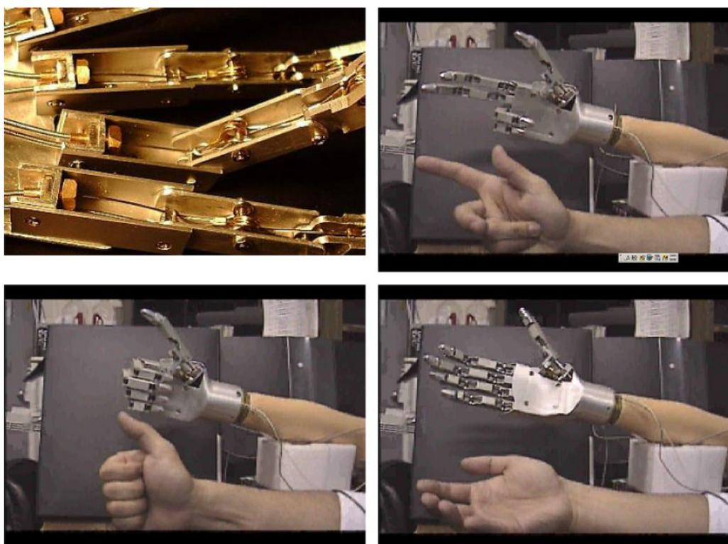
Figure 1 EMG prosthetic hand.
