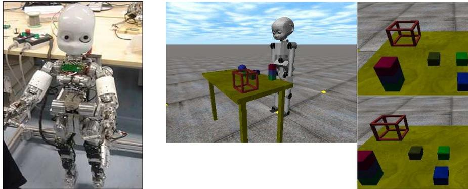
Figure 1: Photo of real iCub (left), of simulated iCub (centre) and of simulated robot's binocular view (right).
