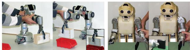
Fig. 18. Set-up of the experiments. Left: KATANA puts a wooden brick into the container, to achieve the task the robot should lift the brick and move it following an elevating trajectory. Right: HOAP-3 grasps a box, to achieve the task HOAP should approach the box with a specific orientation and then lower its arm, as the clench is small, see small figure in the corner.
